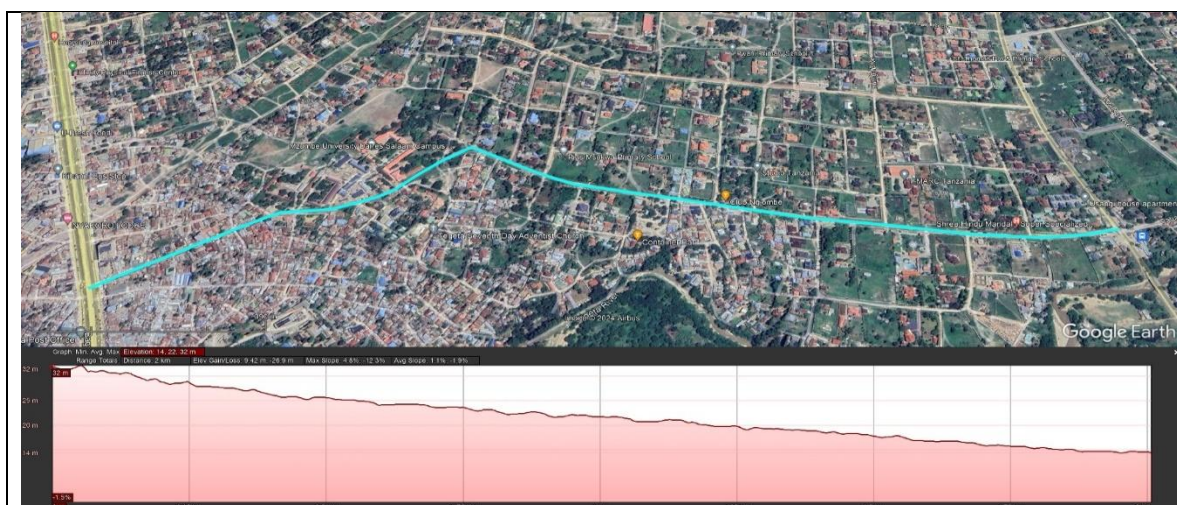
Figure 2.3.4-2: Elevation Profile along Tegeta-Police - Silver Road Section.
