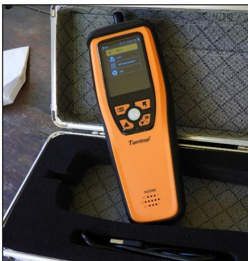
Temtop M2000C device, used for measurement of dust level
