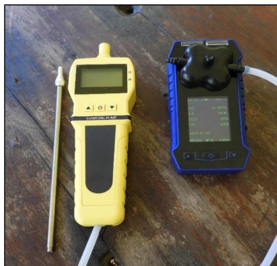
FD-4S Portable Multi-Gas Detector used for measurement of ambient gaseous pollutants.
